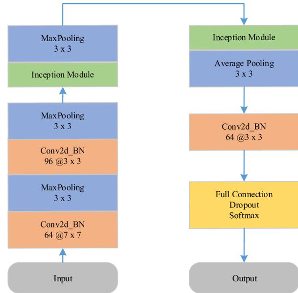
**Figure 4. Architecture of our proposed neural network.**
