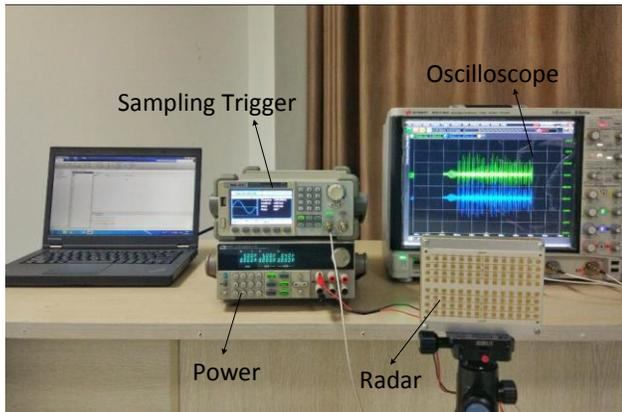
Figure 1. Schematic of the experimental configuration.
